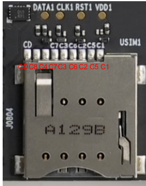
Figure 20: Pin Assignment of (U)SIM Card Connector J0804
